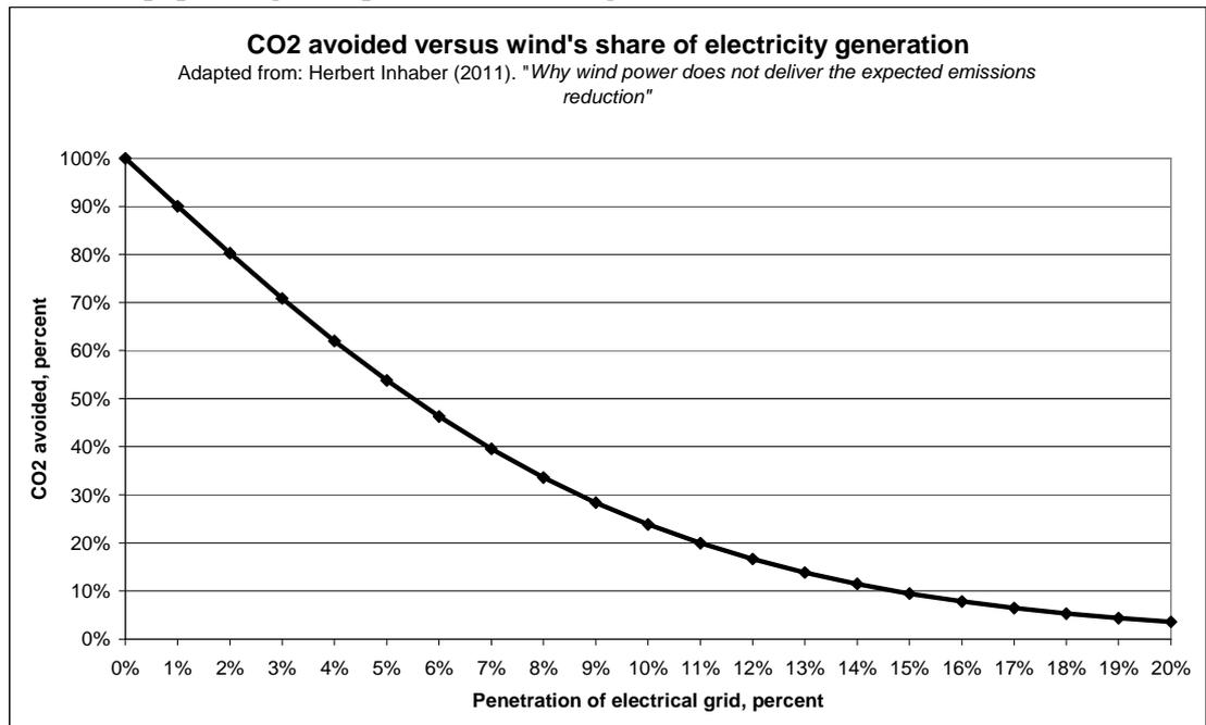
**Fig. 3.** A schematic graph of CO<sub>2</sub> reductions as a function of wind (or other intermittent renewables) penetration into an electrical grid. Penetration is defined as the average fraction of energy contributed by wind to overall energy consumption. [...]
